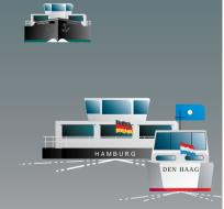
VESSEL DISPLAYING BLUE CONES BY DAY OR BLUE LIGHTS BY NIGHT IS CARRYING DANGEROUS GOODS DO NOT BERTH CLOSER THAN 1 Cone- 10m, 2 Cones- 50m, 3 Cones- 100m DO NOT ATTEMPT TO ENTER A LOCK WITH A VESSEL DISPLAYING 2 OR 3 BLUE CONES
